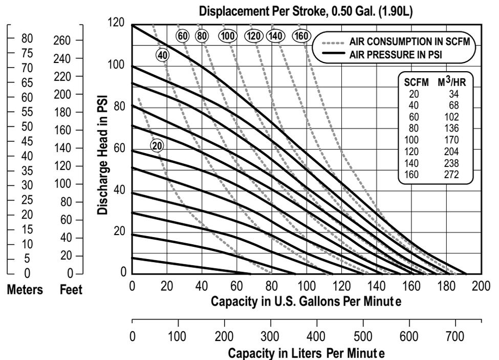
NOTE: For U2 pumps fitted with PTFE diaphragms, reduce water discharge figures by 20%. Suction lift is reduced to 10' (3.05m) dry and 20' (6.10m) wet.
