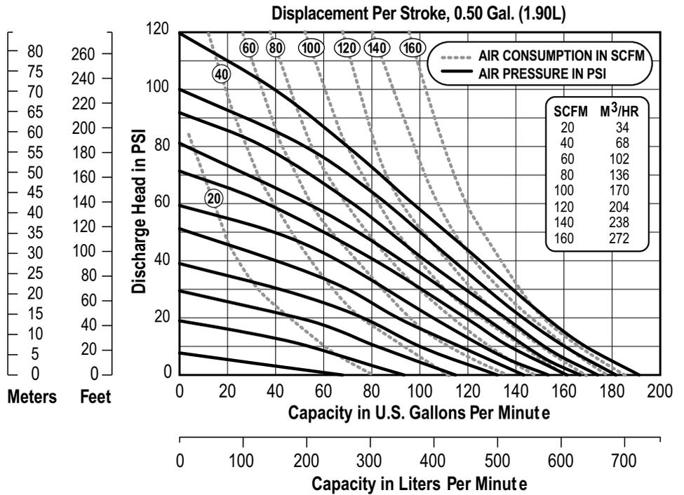
NOTE: For U2 pumps fitted with PTFE diaphragms, reduce water discharge figures by 20%. Suction lift is reduced to 10' (3.05m) dry and 20' (6.10m) wet.
